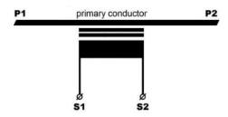
For a transformer with a double ratio:
