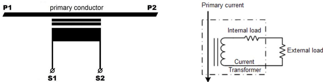
Illustration 1: Wiring diagram current transformer
